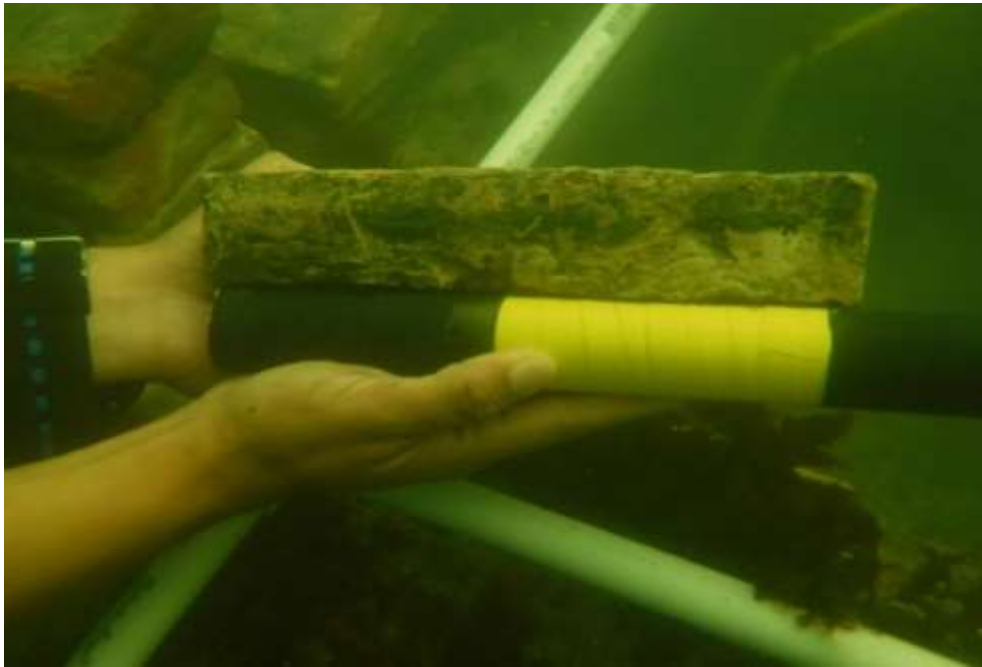
Figure 17. Bricks (21-22 cm in length) with black discoloration (East Carolina University Image)
